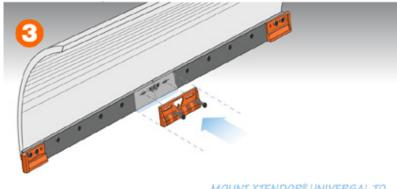
MOUNT XTENDOR® UNIVERSAL TO CENTER OF THE PLOW, HAND TIGHTEN.
