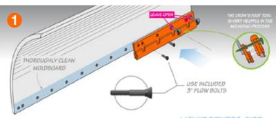
MOUNT DRIVERS-SIDE FIRST USING SHORT 3" BOLTS - HAND TIGHTEN. LEAVE THREE OUTER BOLT HOLES FOR STEP 3
