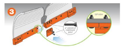
INSTALL CENTER NOSE PIECES WITH 2" GRADE 8 CARRIAGE BOLT. NOTE: NOSE GUARD OVERLAPS END OF BLADE
